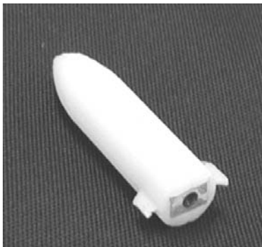
(b) Housing made from FDM
